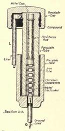
Fig. 172.—The General Electric Company compression-type lightning protector.
